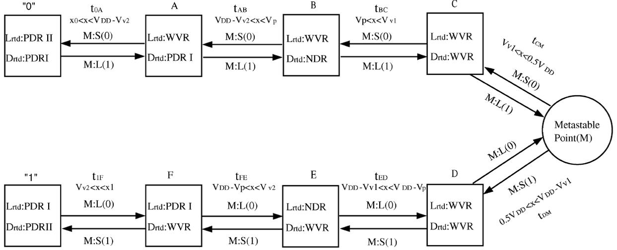
Fig. 4. TRAM WRITE operation microstate diagram.  $L_{rt,d}$  and  $D_{rt,d}$  represent the load RTD and driver RTD, respectively.  $M : S(1)$ ,  $M : S(0)$ ,  $M : L(1)$ , and  $M : L(0)$  represent the saturation ( $S$ ) and linear ( $L$ ) operation region of the access transistor. (1) denotes WRITE "1" operation and (0) denotes WRITE "0" operation.
