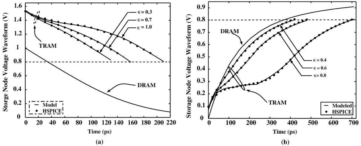
Fig. 6. Storage node waveforms during WRITE operation (a) Write "0" operation. (b) Write "1" operation.
