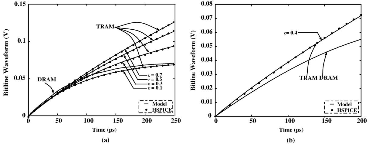
Fig. 5. Bit-line waveforms during READ operations. (a) Read "0" operation. (b) Read "1" operation.
