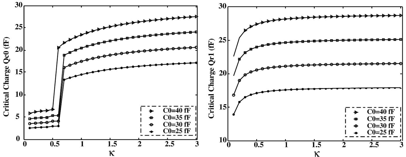
Fig. 7. Critical charge of READ operation with respect to  $\kappa$ . (left) READ “0” operation. (right) READ “1” operation.
