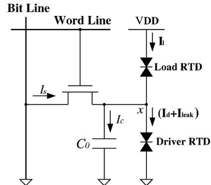
Fig. 1. Schematic diagram of 1T RTD-based RAM.
