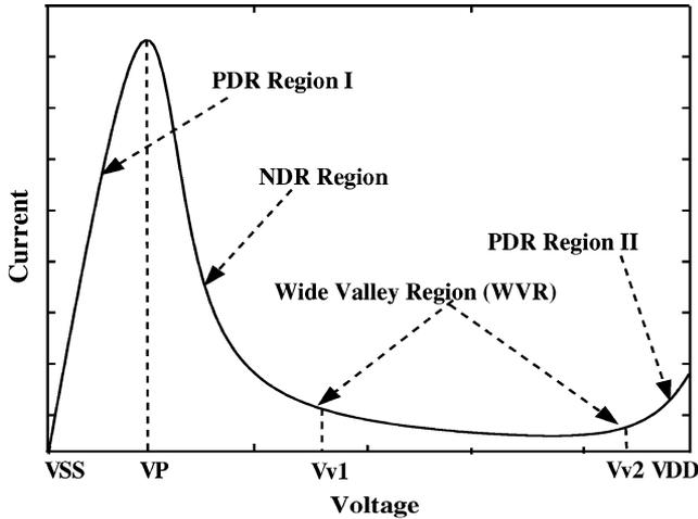
Fig. 2. Typical  $I$ - $V$  characteristic of RTD.
