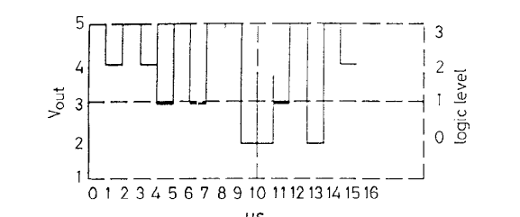
Fig. 17 Simulation results for V_{out} of a 2-input 4-valued logic gate
