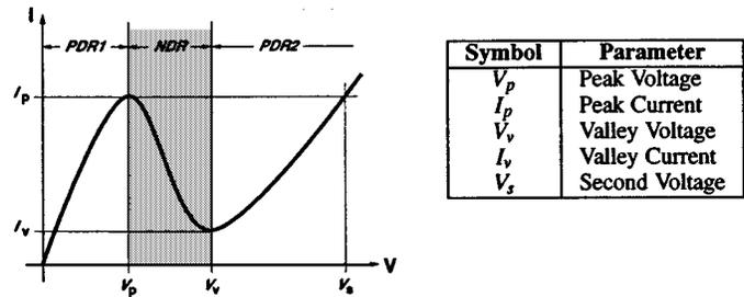
Fig. 1.  $I$ – $V$  characteristic of an RTD.
