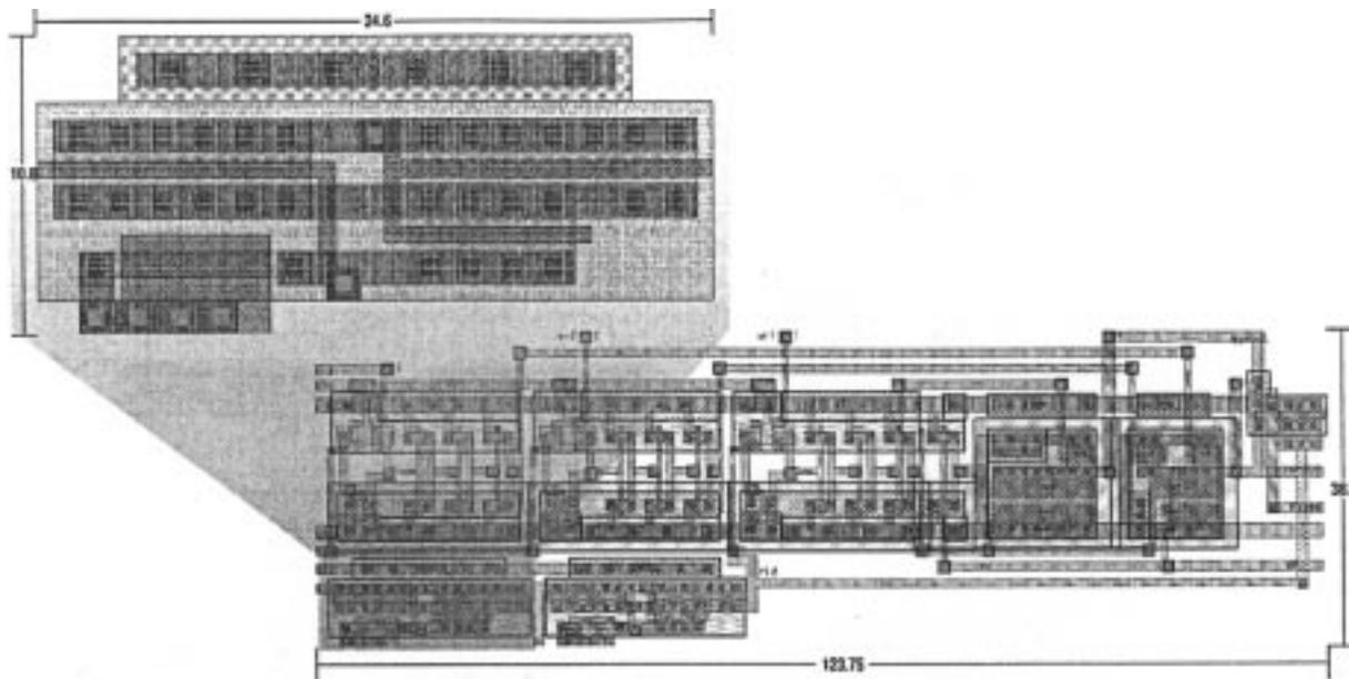
Fig. 10. SDFFA cell layout for a 0.6- $\mu\text{m}$  process. The expanded block corresponds to the MOS-NDR subcircuit. Dimensions are noted in micrometers.
