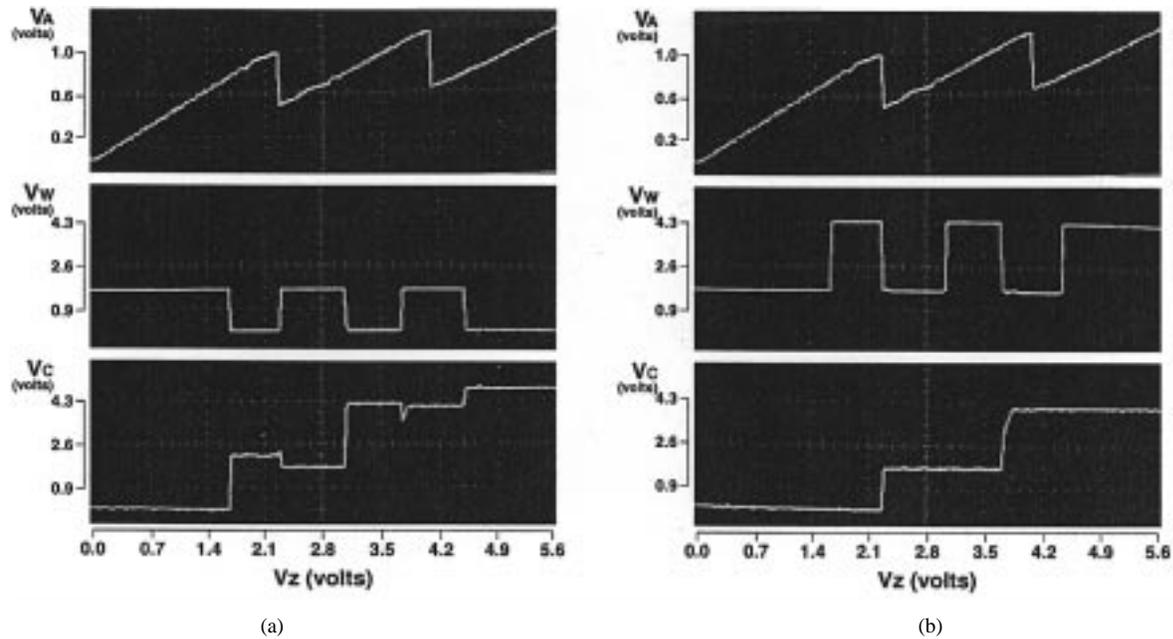
Fig. 12. Measured results at low speed showing the transfer characteristics of the SDFA cell. (a)  $InZ_1 = L$ . (b)  $InZ_1 = H$ .
