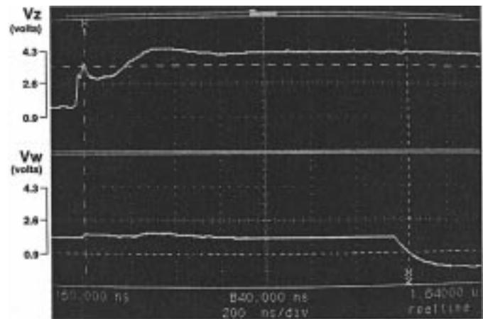
Fig. 13. Measurement of worst case gate delay, including delay of the chip pads.
