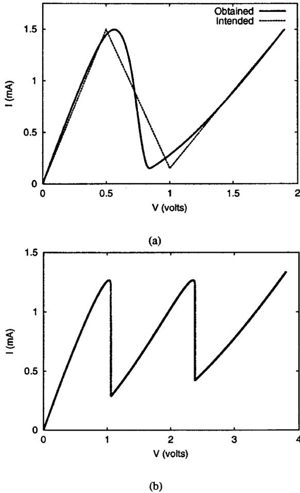
Fig. 8. (a) Simulated  $I$ - $V$  characteristics of the sized NDR circuit. (b) Two-peak current-voltage characteristics of two MOS-NDR circuits connected in series with applied  $V_{gg}$  of 4 and 4.25 V.
