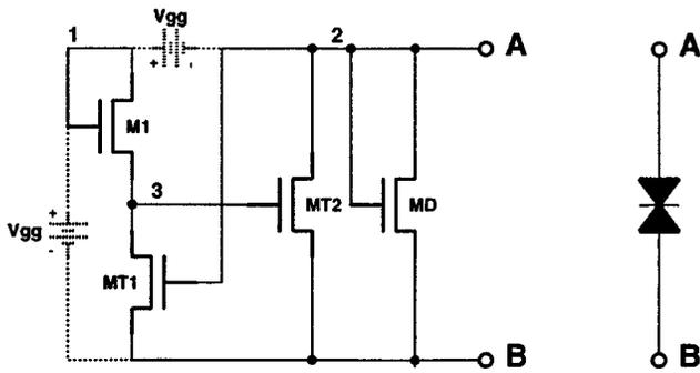
Fig. 6. The four-transistor MOS-NDR circuit emulates the RTD  $I$ - $V$  characteristics. Two possible ways of applying  $V_{gg}$  are shown.
