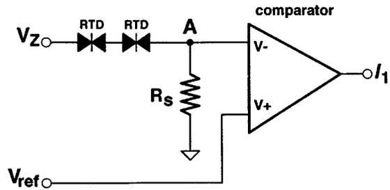
Fig. 4. Compact circuit for implementing literal  $l_1$ .
