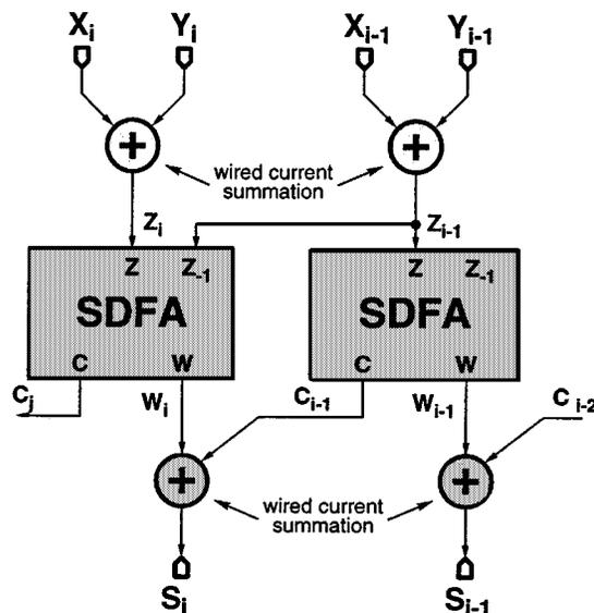
Fig. 2. Scheme for parallel addition using the signed-digit full adder (SDFA) cell.
