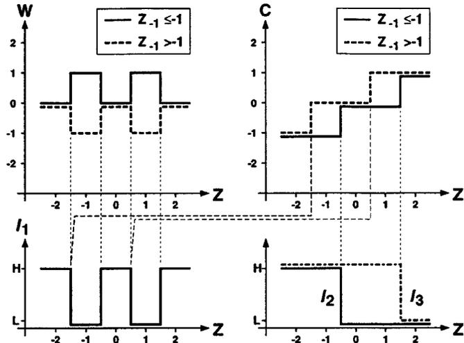
Fig. 3. SDFA block output functions and their description by means of three literal signals  $l_1$ ,  $l_2$ , and  $l_3$ .
