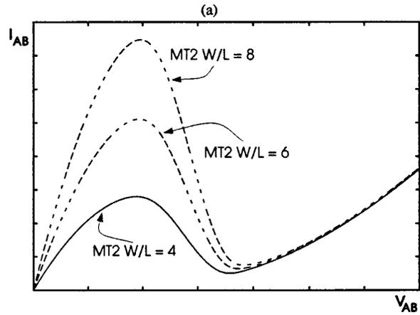
Fig. 7. Simulation results showing the effect of varying  $W/L$  of (a) *MT1* and (b) *MT2* while holding  $V_{gg}$  constant.
