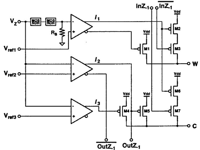
Fig. 9. S DFA cell circuit schematic diagram.
