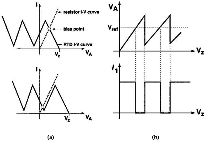
Fig. 5. (a) The load-line method is used to describe the behavior of the voltage at node *A*. (b) Generation of literal  $I_1$  by comparison of voltage  $V_A$  to reference voltage  $V_{ref}$ .
