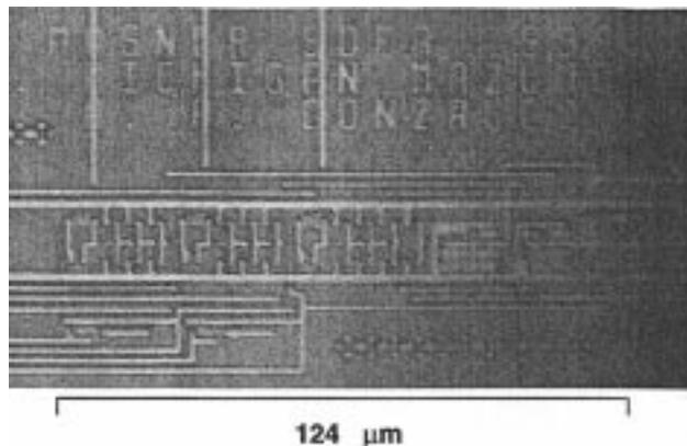
Fig. 11. Chip microphotograph of fabricated signed-digit adder prototype.
