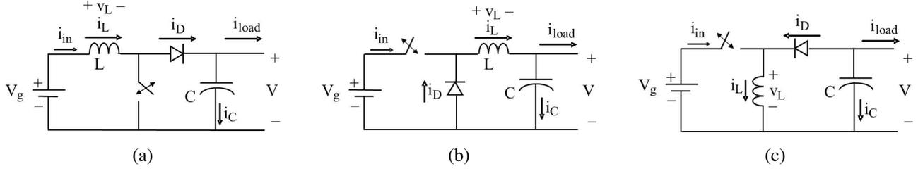
Fig. 2: Circuit representing (a) Boost converter, (b) Buck converter, and (c) Buck-Boost converter. Note that  $i_{load}$  includes both the nominal load current, as well as ripple current. The converters are assumed to operate in continuous-conduction-mode (CCM). Boost converters step up the voltage at the output, while buck converters step down the voltage. A buck-boost converter can achieve both the objectives.
