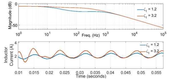
Fig. 9: Bode plots of inner-shaped plants  $\tilde{G}_c$  and inductor currents for different  $\zeta_1$ . While the average (or DC) current remains the same as desired, the smaller values of  $\zeta_1$  result in relatively smaller magnitudes of 120 Hz ripple in inductor currents.
