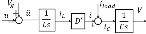
Fig. 3: Block diagram representation of a boost-type converter. The control signal  $\tilde{u}$  is converted to an equivalent PWM signal to command the gate of the transistor acting as a switch.
