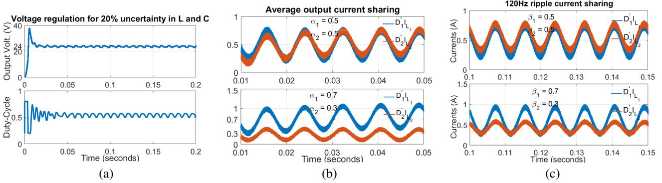
Fig. 8: (a) Voltage regulation in presence of modeling uncertainties and 120 Hz ripple at the output. The inner-outer controller regulates the output voltage to the desired voltage,  $V_{des} = 24V$ . (b) Average current (power) sharing between two converters in the ratios 1 : 1 and 7 : 3. (c)  $\omega_0$  average ripple sharing between two converters in the ratios 1 : 1 and 7 : 3.
