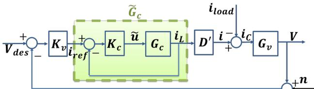
Fig. 4: Block diagram representation of the inner-outer control design. Exogenous signals  $V_{des}$  and  $i_{load}$  represent the desired output voltage and disturbance, respectively. The quantities  $V$  and  $i_L$  represent the available measurements.
