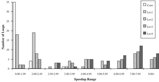
Figure 10: Speedup distribution for an issue-8 superscalar/VLIW processor.
