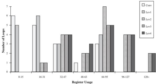
Figure 13: Register usage distribution of DOALL loops only for an issue-8 superscalar/VLIW processor.
