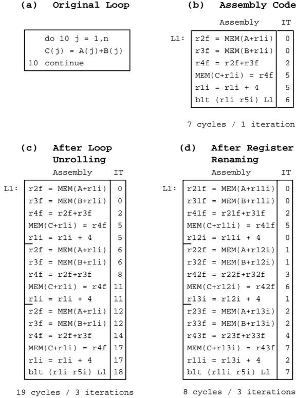
Figure 1: Example of loop unrolling and register renaming. All examples in this paper assume a superscalar processor with infinite resources and no register renaming hardware. Also, the issue times (IT) shown are for the code after code scheduling but in order to preserve clarity, the unscheduled code is shown. Sorting by issue time yields the scheduled code.
