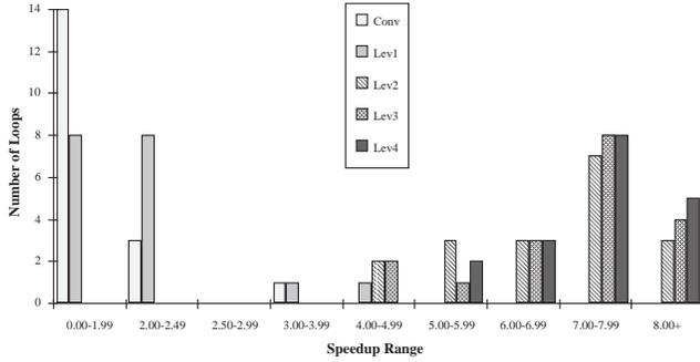
Figure 12: Speedup distribution of DOALL loops only for an issue-8 superscalar/VLIW processor.
