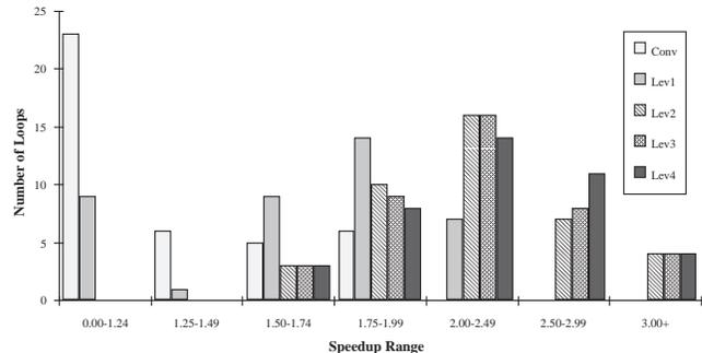
Figure 8: Speedup distribution for an issue-2 superscalar/VLIW processor.
