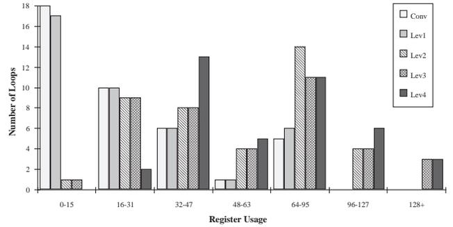
Figure 11: Register usage distribution for an issue-8 superscalar/VLIW processor.
