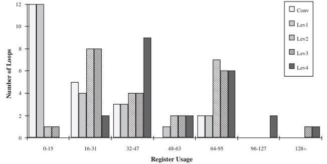
Figure 15: Register usage distribution of non-DOALL loops only for an issue-8 superscalar/VLIW processor.
