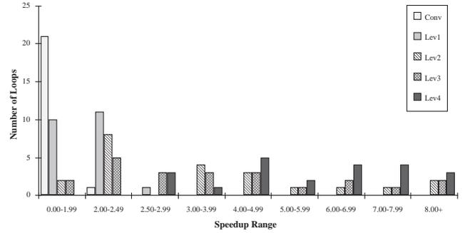
Figure 14: Speedup distribution of non-DOALL loops only for an issue-8 superscalar/VLIW processor.
