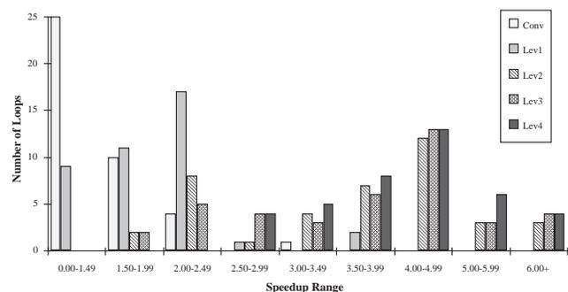
Figure 9: Speedup distribution for an issue-4 superscalar/VLIW processor.
