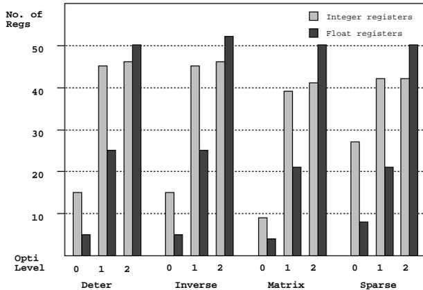
Figure 5: Maximum register usage across register preload support levels.
