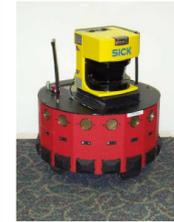
Experiments were performed with Lassie, an RWI Magellan Pro mobile robot, using a laser range finder scan for an image. The laser range finder returns 180 range points in a half-circle in front of the robot. Lassie does not have a compass.
