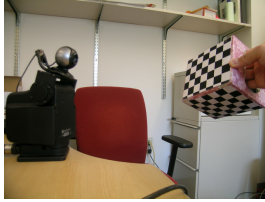
Fig. 3. A box is moving around in front of a webcam mounted on a pan tilt unit.
