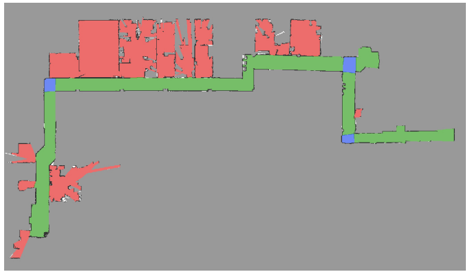
Figure 4: Metric-topological map of the demonstration environment. This 44m x 75m map was produced by running Vulcan’s metric SLAM and place classification algorithms on sensor data of the wheelchair being manually driven through an environment. Color indicates the “type” of each region in the topological map: decision points are blue, path segments are green, and destinations are red.
