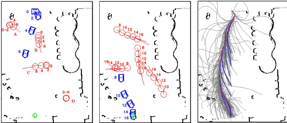
Fig. 8. (Best viewed in color) Robot motion in the same environment as Fig. 7, but with low weights on the action cost ( $c_3 = 0.04$  and  $c_4 = 0.02$ ). The robot moves more aggressively and cuts in front of the dynamic object marked C, which it passed behind in Fig. 7. **Left and Center:** Time-stamped snapshots of the robot and pedestrian. **Right:** Trajectories sampled by the planner (gray), time-optimal plans selected at each planning cycle (blue) and the actual path taken (red).
