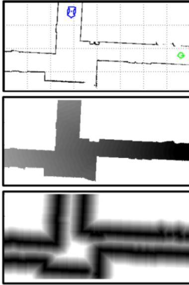
Fig. 3. The information about the static world available to the robot. **Top:** Occupancy grid map ( $20 \times 10\text{m}$ ) with initial robot pose (blue) and the final goal (green circle). **Middle:** Navigation function. **Bottom:** Proximity to walls.
