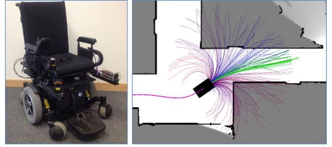
Fig. 2. (Best viewed in color) **Left**: Differentially driven wheelchair robot (0.76m x 1.2m), equipped with laser range finder and SLAM capability. **Right**: Sampled trajectories parametrized by  $z_*$  (19), generated by a dynamically simulated vehicle operating under the stabilizing control policy (15)-(18) in a SLAM-generated map. The wheelchair is depicted as a black rectangle. Green to red color gradient indicates low to high expected navigational cost (21). See text for details.
