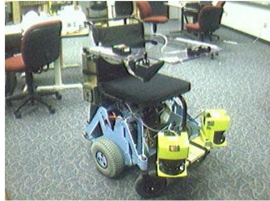
Figure 1. The wheelchair robot has a stereo camera and two laser range-finders.
