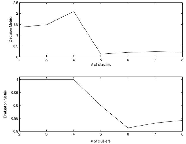
Figure 3: After Lassie explores the notched rectangle,  $k = 4$  is selected as the best number of clusters by the decision metric  $M$  (top), and is confirmed as optimal by the evaluation metric  $U$  (bottom).
