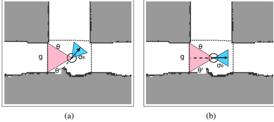
Figure 7.2: (a) shows the angle subtended by gateway  $g$  relative to the the agent, drawn as a circle with the arrow indicating its heading. The blue cone on the right shows the estimated heading  $\mu_\theta$  and along with a  $1\sigma$  bound. In this case,  $\theta$  and  $\theta'$  are on the same side of the dashed wraparound line. The other possible scenario is shown in (b), where  $\theta$  and  $\theta'$  are on opposite sides of the wraparound at  $\pi$ .
