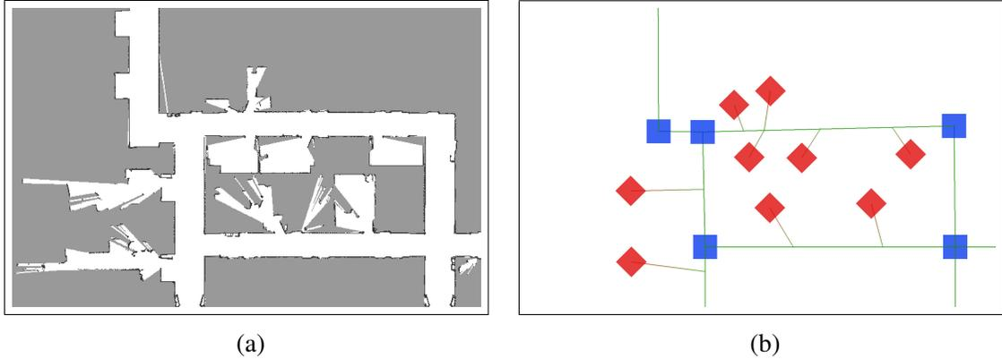
Figure 1.1: (a) shows the occupancy grid of a typical office environment. The corresponding  $H^2SSH$ -style topological map of the building is shown in (b). The lines are path segments, the squares are decision points, and the diamonds are destinations, each office is a single destination connected to its adjacent hallway.
