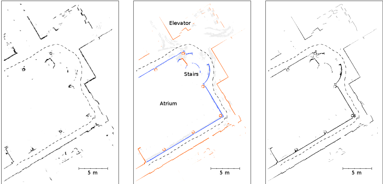
(a) Traditional occupancy grid mapping of the environment in Figure 1 (LIDAR sensor path shown as dashed line) produces a map in which most of the highly transparent glass walls are entirely missing, giving the illusion of navigable free space across the atrium. (Only 13% are correctly detected, mostly small regions of glass near the spiral staircase, which are visible due to subtle optical effects, refer to Section III-A.2). The shiny metal doors of the elevator are also missing, showing that the problem is general to other non-diffuse materials as well.
