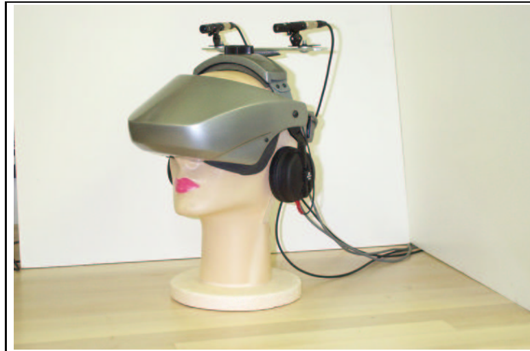
Figure 8. Video See-Through Augmented Reality with a 5DT HMD and two Sony Lipstick cameras.
