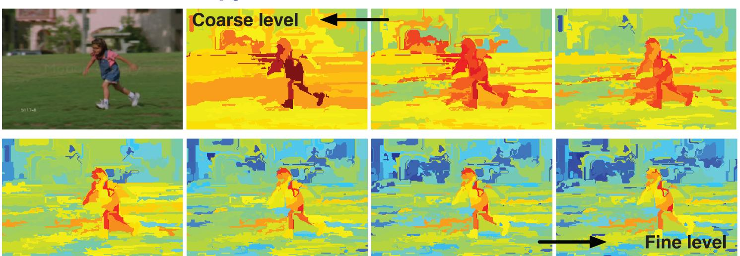
Node entropy in a hierarchy for the motion feature criterion
