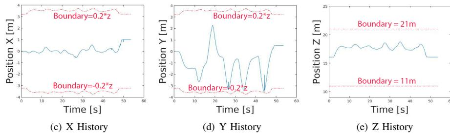
Fig. 3. Position history of real flight under perfect measurements and no disturbance compensation.
