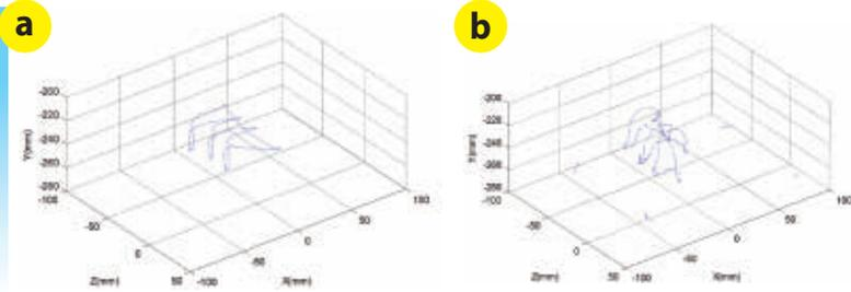
**FIGURE 5** Tool tip trajectory in 3-D space (a) Autonomous Operation The trajectory of four peg board markers has little movement due to dedicated tool-object interaction (b) Human Teleoperation The trajectory of four peg board markers shows large movement due to tool collision.
