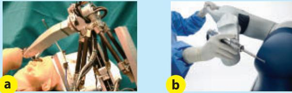
**FIGURE 2** Examples of cooperative robots: (a) The JHU REMS robot for head & Neck microsurgery [4]. (b) the Mako Rio@ for orthopedic surgery.
