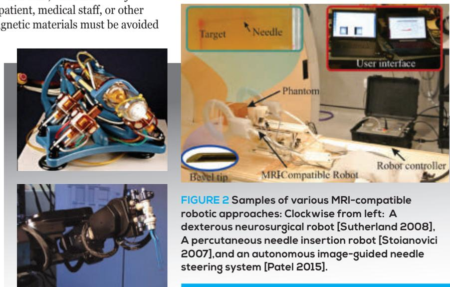
**FIGURE 2** Samples of various MRI-compatible robotic approaches: Clockwise from left: A dexterous neurosurgical robot [Sutherland 2008], A percutaneous needle insertion robot [Stoianovici 2007], and an autonomous image-guided needle steering system [Patel 2015].
