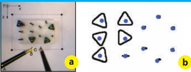
**FIGURE 4** Computer Vision Tool and object detection: (a) Locations of markers (Points A, B) on the surgical tool as acquired by the stereo camera for predicting the location of the tool tip (Point C); (b) Top view computer vision detection of the set of pegs tips (dots) and the triangular shaped block.
