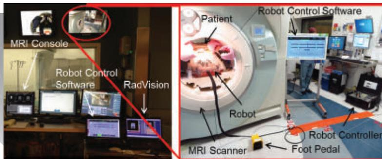
**FIGURE 3** An example of a clinical configuration for MR image-guided prostate cancer biopsy using the robot described in [Eslami 2015].
