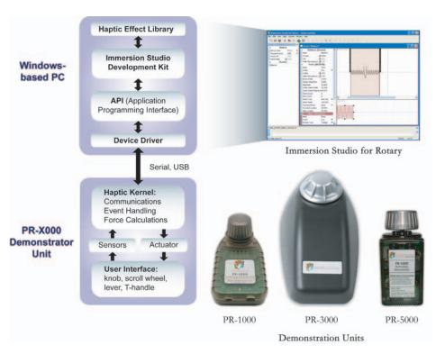
Similar to the Runtime System Architecture, haptic effects created by Immersion Studio for Rotary software are sent by the Rotary API through the device driver to the demonstration unit so designers can immediately experience their haptic creations.
