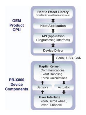
TouchSense modules use a position sensor, actuator, amplifier, microprocessor with firmware controls, and push-to-select (PTS) switch to provide precise and reliable response that won't degrade over time.
