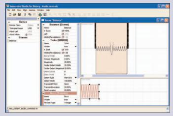
Immersion Studio for Rotary software provides an easy-to-use graphical user interface for creating haptic effects. When triggered, a time-based effect (periodic) shown in the bottom frame will play for a set period of time. A position-based event, such as the one shown in the top frame, will play as the user rotates the rotary module. The scene property window on the left allows designers to change all haptic parameters including amplitude, start position, width, duration, and shape.
