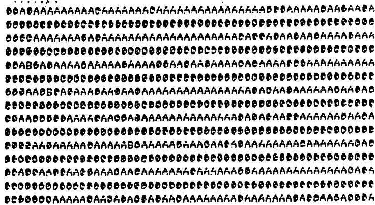
Fig. 6 I-V map of an array section 47 mm X 5.4 mm, (810 elements), where "@,A,B,C,D,*" represent different diode breakdown voltages.
