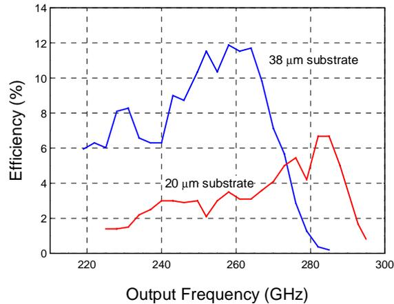
**Figure 9. Triplers of nominal 280 GHz design fabricated on different thicknesses of GaAs. The difference in efficiency is probably due to the quality of the diodes, while the frequency shift is due to substrate thickness.**
