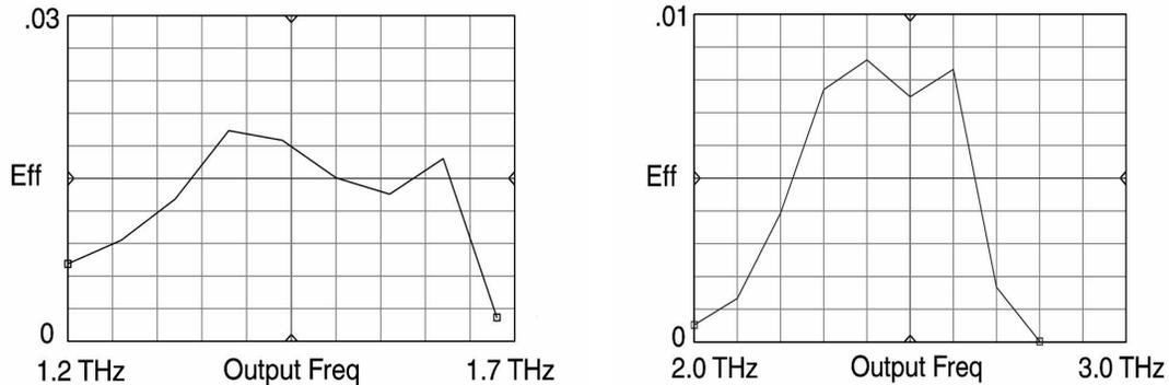
**Figure 10. Predicted bandwidth of balanced doublers in two bands to test the feasibility of THz multipliers. The efficiency scale is largely arbitrary, since almost nothing is known about multiplier performance at these frequencies.**
