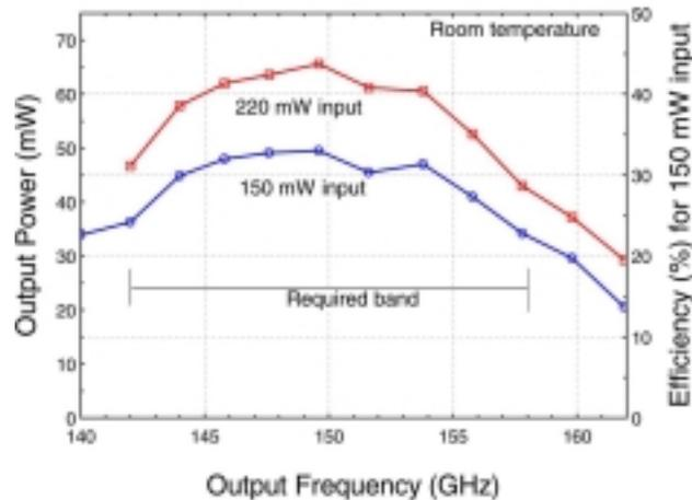
**Figure 1. Frequency response of balanced doubler built to demonstrate one of the driver bands for FIRST. The efficiency corresponds to the lower curve.**
