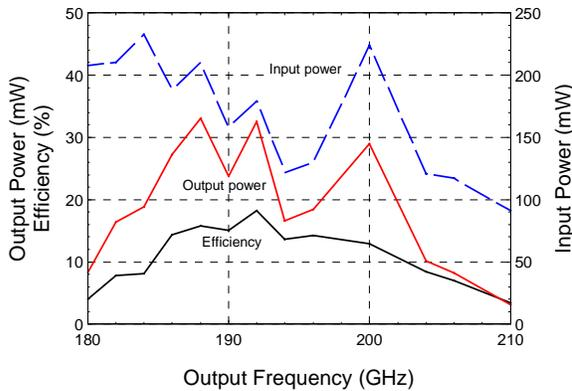
**Figure 3. Frequency response of doubler with input power as noted.**
