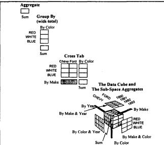
Figure 2: The CUBE operator is the N-dimensional generalization of simple aggregate functions. The 0D data cube is a point. The 1D data cube is a line with a point. The 2D data cube is a cross tab, a plane, two lines, and a point. The 3D data cube is a cube with three intersecting 2D cross tabs.
