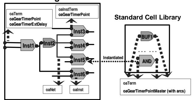
The timing information is stored using the OpenAccess extension mechanism (oaGearTimerPoint, ...)
