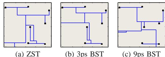
Fig. 1. Min-wirelength trees with zero and bounded skew (Elmore delay). Only fragments of actual clock trees are shown.
