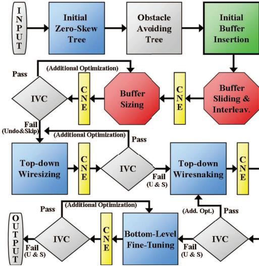
Fig. 2. Key steps of the Contango methodology. Blue boxes represent *skew reduction* techniques, red octilinear shapes show *CLR reductions*, and the green box with thick border reduces both objectives. An Improvement- & Violation-Checking (IVC) step follows each Clock-Network Evaluation (CNE) using circuit simulation tools, e.g., SPICE. “Fail” indicates no improvement or having slew violations, leading to a transition to the next optimization.
