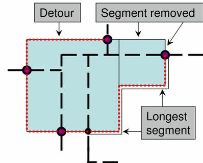
Fig. 3. An illustration of our detouring algorithm. Small solid circle indicates the source of detour, larger circles indicate sinks. The detour is shown with red dotted lines.
