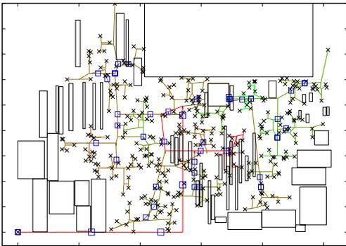
Fig. 4. The clock tree produced by Contango on *ispd09fnb1*. Sinks are indicated by crosses, buffers are indicated by blue rectangles. L-shapes are drawn as “diagonal wires” to reduce clutter. Wires are colored by a red-green gradient to reflect slow-down slacks, as described in Section III-B. The impact of wiresnaking is too small to be visible.
