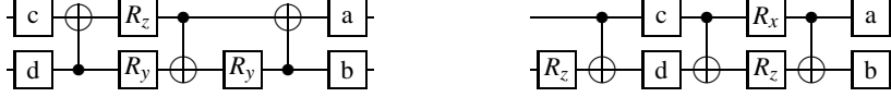
Figure 2. Universal two-qubit circuit with three CNOT gates, and a total of 10 basic gates. 3 The left circuit requires 18 gates from \{\text{CNOT}, R_y, R_z\} , whereas the right circuit requires 18 gates from \{\text{CNOT}, R_x, R_z\} .
