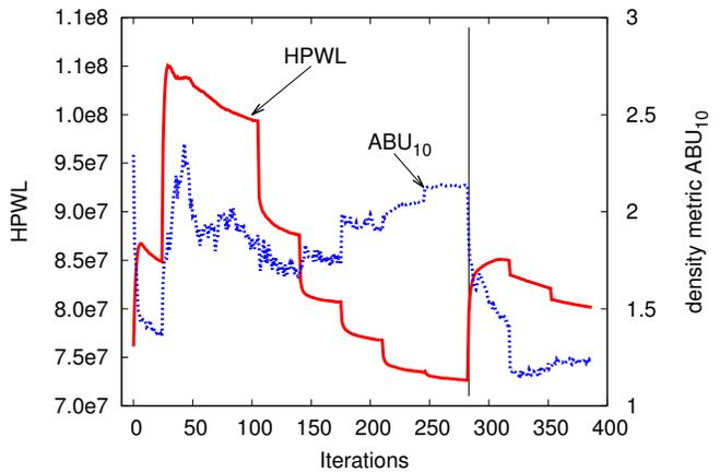
**Figure 1: Progressions of wirelength and the density metric  $ABU_{10}$  over ILR iterations on ADAPTEC1. Unclustering is marked with a vertical line. ILR disruptively improves  $ABU_{10}$  and increases the wirelength. Each ILR iteration traverses all movable modules once.**
