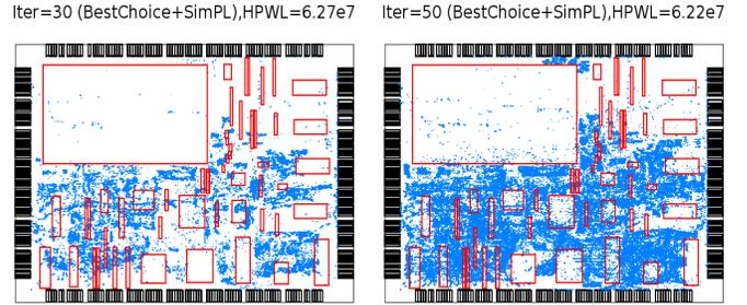
**Figure 5: Macro placement on NEWBLUE1. (left) Macros are fixed at top-level placement iteration 30. (right) Further iterations optimize cell locations.**
