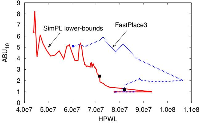
**Figure 3: Progression of the density metric  $ABU_{10}$  versus wirelength, comparing SimPL lower-bounds (w/ FastPlace-DP) and FastPlace3 on ADAPTEC1. Steeper slope and datapoints closer to the origin indicate better trade-offs. Each square box indicates the beginning of detailed placement.**
