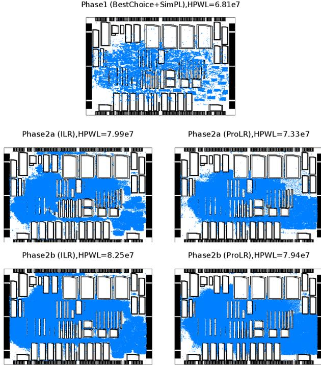
**Figure 6: Snapshots of global placement (ADAPTEC1) after each phase of Algorithm 1 for MAPLE with ILR (left) and MAPLE with ProLR (right). Phase1 is top-level placement (BestChoice+SimPL). Phase2a and Phase2b perform LR placement of the coarsened and flat netlist, respectively.**
