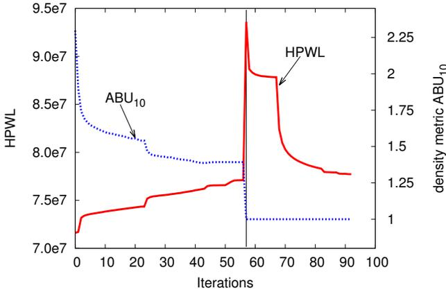
**Figure 2: Progressions of wirelength and the density metric  $ABU_{10}$  over FastPlace-DP iterations on ADAPTEC1. The start of detailed placement is marked with a vertical line. Placements with high utilization undergo significant changes as full legalization completes.**
