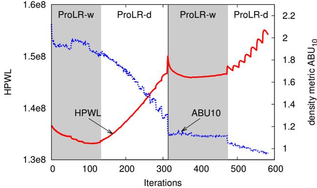
**Figure 4: Progressions of wirelength and the density metric  $ABU_{10}$  over ProLR iterations (BIGBLUE2). Unclustering is marked with a vertical line. ProLR alternates ProLR-w (shaded) and ProLR-d phases.**
