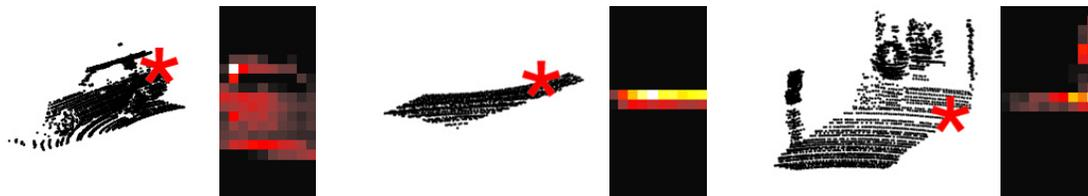
Figure 3.1: Three example pairs of point clouds (a car, a road, and a ground with non-car objects) and the corresponding spin-images. Left of each pair: A view of a point cloud produced by the laser range finder. Right of each pair: A spin-image generated around the point marked with a red star on the left.
