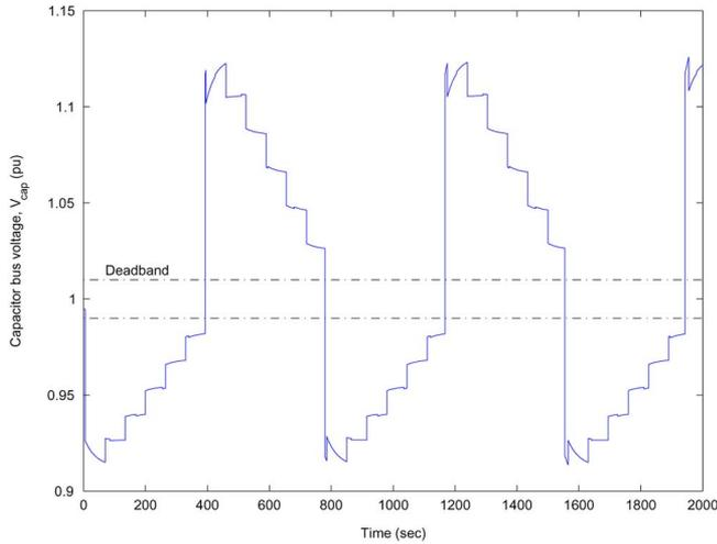
Fig. 5. Capacitor voltage trajectory.
