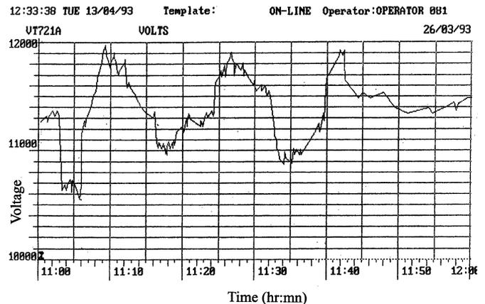
Fig. 1. Oscillations observed in a distribution system.
