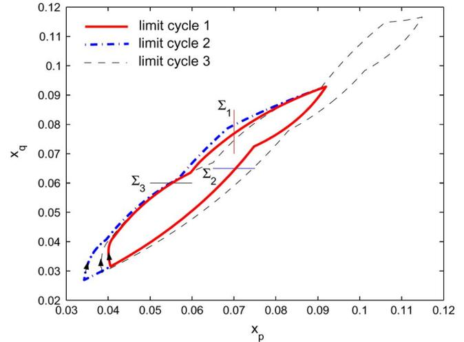
Fig. 11. Different Poincaré hyperplanes locating different limit cycles.
