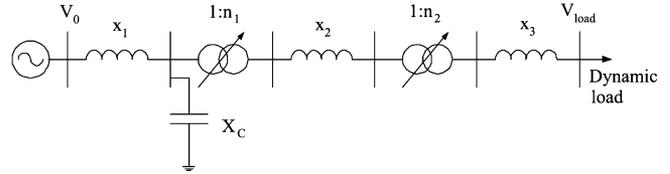
Fig. 7. System of cascaded transformers feeding a dynamic load.
