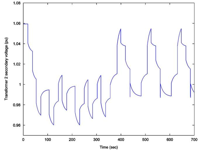
Fig. 8. Load-side voltage for the cascaded transformer system.
