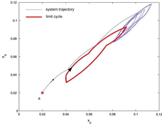
Fig. 9. State-space behavior of the cascaded transformer system, shown in the  $x_p - x_q$  plane.
