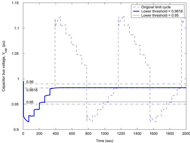
Fig. 3. Influence of deadband lower limit  $V_{\min}$  on behavior.
