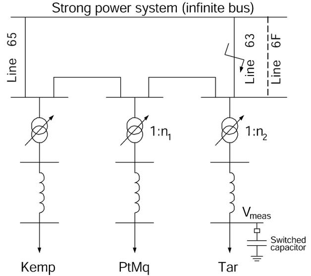
Fig. 2. Supply system (simplified) one-line diagram.
