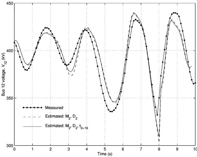
Fig. 5. Comparison of voltage recording with estimated model behavior.
