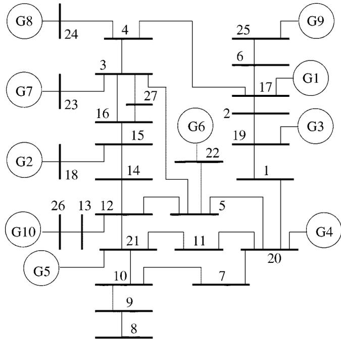
Fig. 1. Nordel system model.
