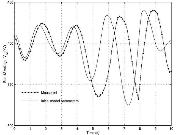
Fig. 3. Comparison of voltage recording with initial model behavior.
