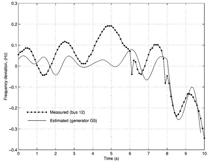
Fig. 6. Comparison of frequency recording with estimated model behavior.
