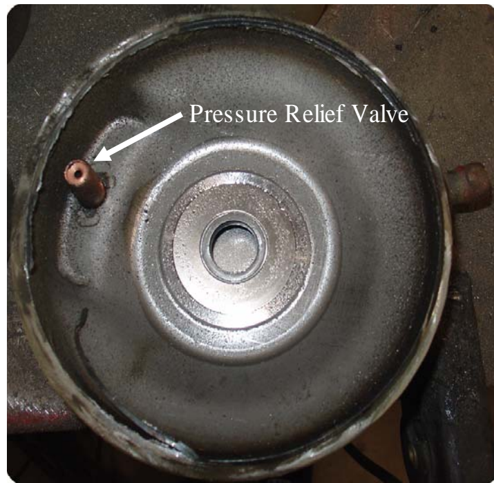
Figure 7 Pressure Relief Valve
