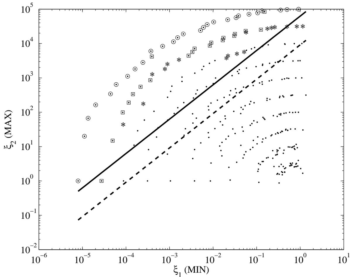
Figure 15: *Three first Pareto fronts (o, □ and \*) and boundaries of paired t test acceptance regions for the scattergram of Fig. 14.*
