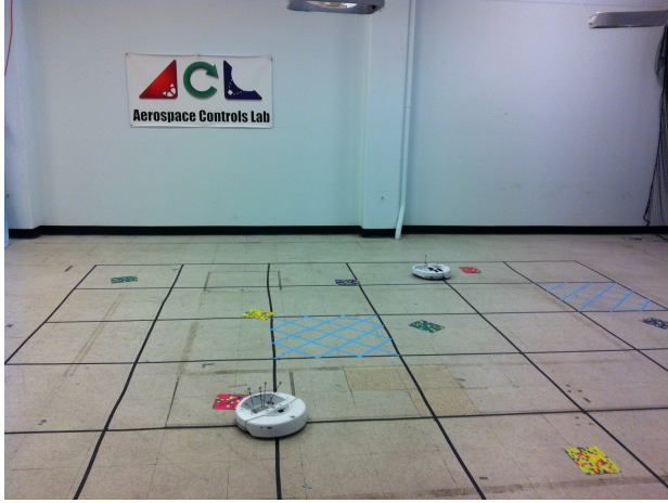
Figure 2: Hardware testbed in Aerospace Controls Lab., MIT. Targets are patched pictures glued on ground, with dominant color representing its classification. Exploration is done by security cameras hanging on the wall. Tasking is done by robots visiting targets.
