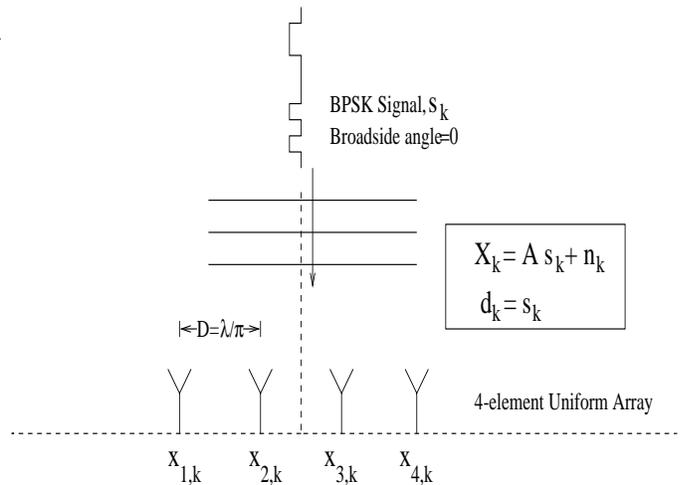
Fig. 1. Signal Scenario for Example 1
