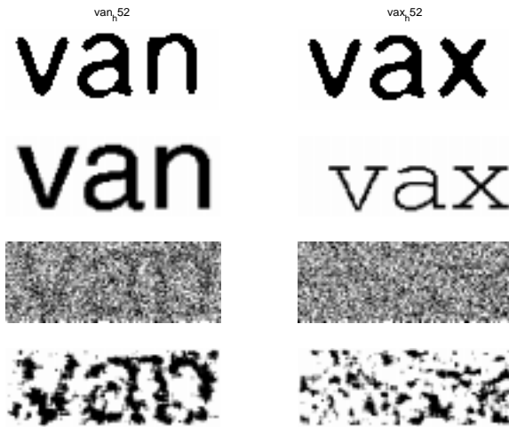
Figure 4. Row 1: van and vax in Helvetica 52. Row 2: van in Helvetica 64 and vax in Courier 52 with random translation. Row 3: row 2 corrupted with noise. Noise level corresponds to maximum noise level of 1 displayed on horizontal axis of Figures 3 and 3. Row 4: row 3 denoised by median filtering with a 7 \times 7 window.
