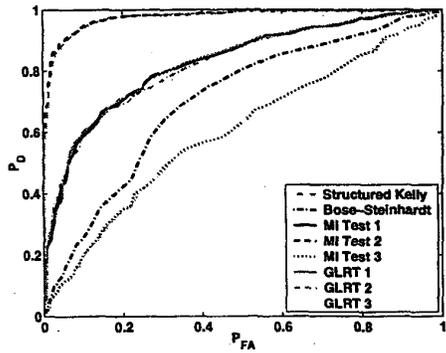
Fig. 7. ROC curves for Case 2 with SNR = 10dB ( $m_A = 50, m_B = 50, n = 61$ ).
