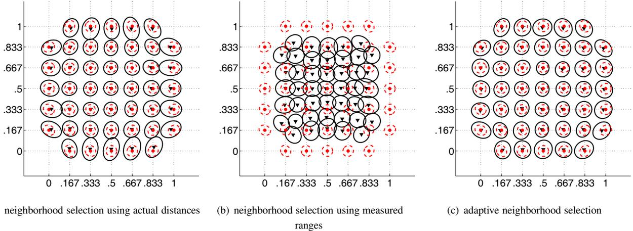
**Fig. 2.** Estimator mean ( $\blacktriangledown$ ) and  $1\text{-}\sigma$  uncertainty ellipse ( $\text{---}$ ) for each blindfolded sensor compared to the true location ( $\cdot$ ) and CRB on the  $1\text{-}\sigma$  uncertainty ellipse ( $\text{- - -}$ ).
