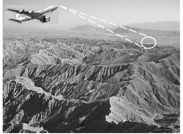
Fig. 1. An illustration of the model problem. A moving sensor is to best choose the waveform and pointing direction to detect and track a ground target. Visibility between the sensor and ground affects one waveform but not the other.
