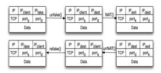
Figure 4: Packet transformations when  $[IP_{client}, port_s]$  tries to connect to  $[IP_{dest}, port_d]$ . The client and the destination perceive the other end to be  $[IP_{fake}, port_d]$  and  $[IP_{exit}, port_k]$  resp.
