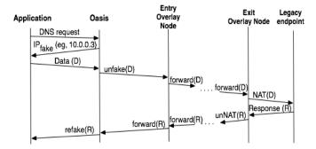
Figure 3: Name-faking based packet timeline
