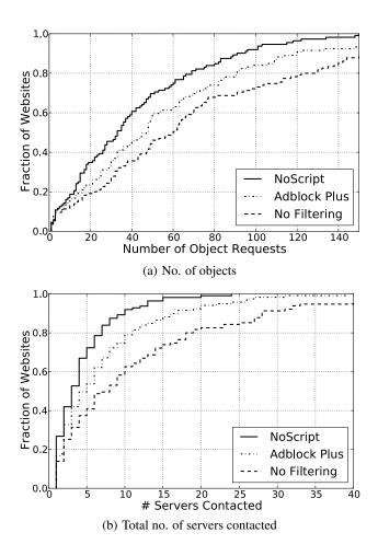
Figure 21: Reduction in number of objects and servers contacted with client-side filtering.
