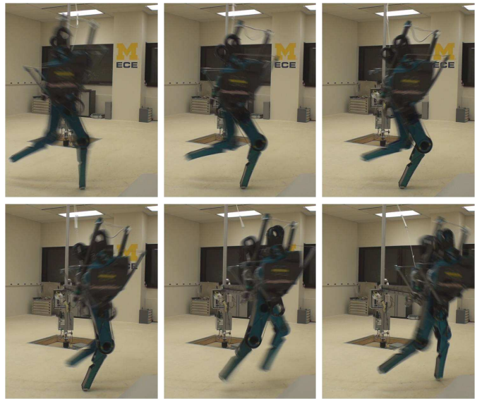
Fig. 5. A typical running step for MABEL. Snapshots are at intervals of 100 ms. The snapshots progress temporally from left to right and from top to bottom. A video of the running experiment is available on YouTube [14].
