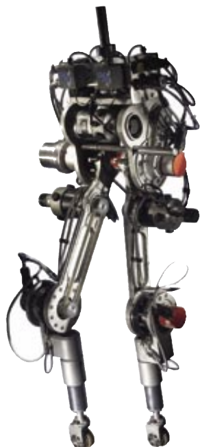
The two-legged robot called RABBIT walks in a manner similar to a human.
