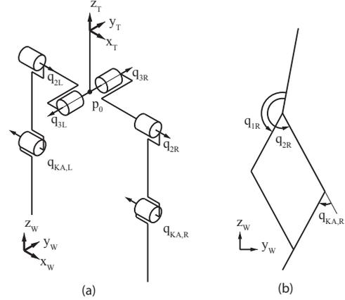
Fig. 2: Mechanical structure and coordinates for MARLO. (a) Conceptual diagram of rigid body model. (b) Each leg is physically realized by a four-bar linkage. The knee angle  $q_{KA,R}$  is related to the angles of the upper links as  $q_{KA,R} = q_{2R} - q_{1R}$ .
