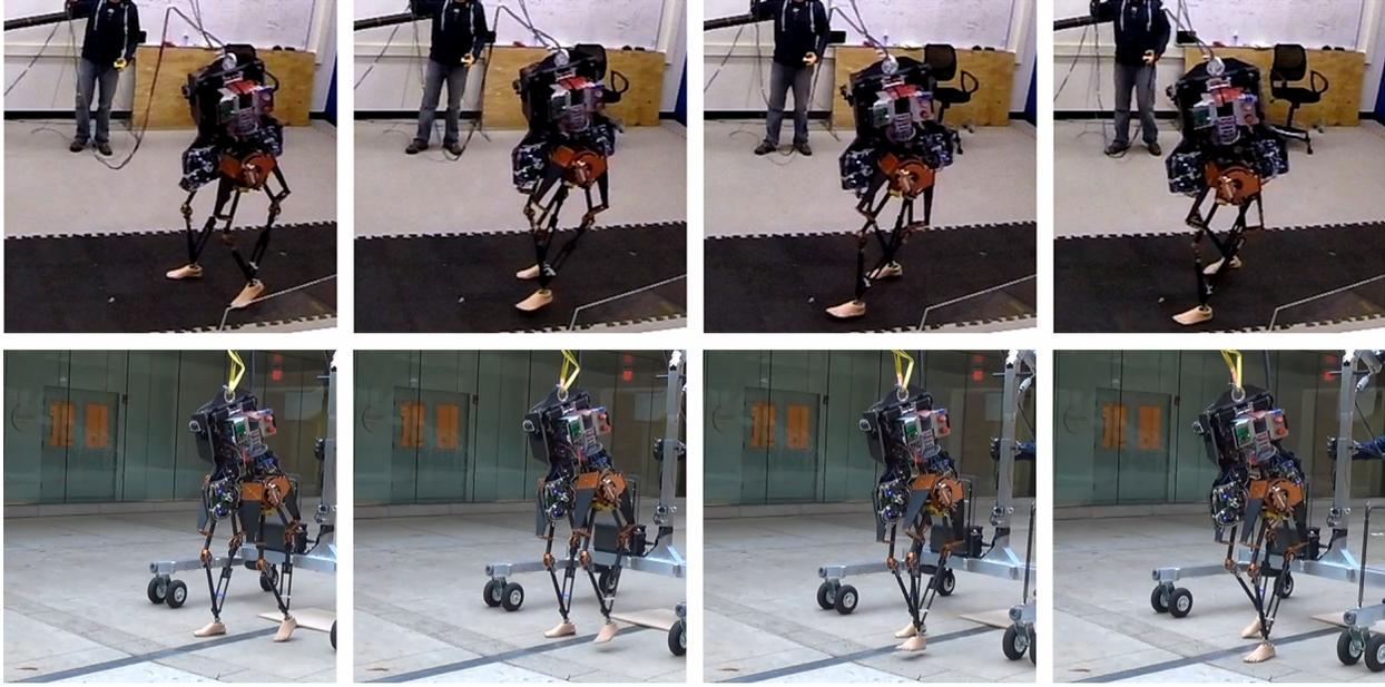
Fig. 6: Video snapshots from two 3D walking experiments. Frames are 200 ms apart. Videos of indoor (top row) and outdoor (bottom row) experiments are available online [28].
