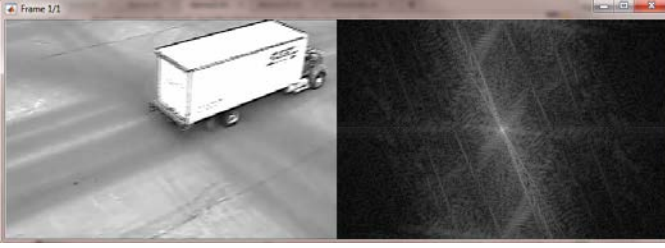
Fig 6 2-D FFT of a frame when there is a vehicle
