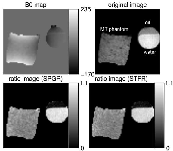
Figure 5.4.4: The  $B_0$  map and the resulting images of Phantom experiment III. Upper-left:  $B_0$  map; upper-right: the original SPGR image with FSMT part off where oil, water and the MT phantom are labeled; lower-left: the ratio image of SPGR taken between the one with FSMT contrast and the one without; lower-right: the ratio image of STFR. These two sequences show similar performance on suppressing fat and producing MTC.
