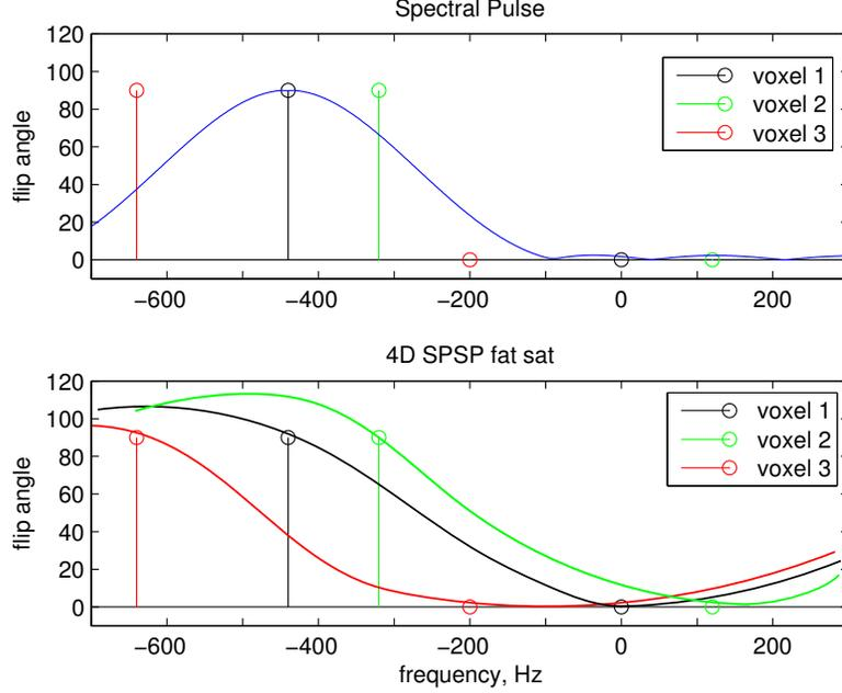
Figure 4.2.1: Illustration of the frequency responses of the SLR fat sat pulse (top) and the 4D fat sat pulse (bottom) in the presence of  $B_0$  inhomogeneity, where 3 voxels at different off-resonance frequencies are selected as examples. The 4D fat sat pulse suppresses fat without exciting water much more effectively with less sharp transition bands.
