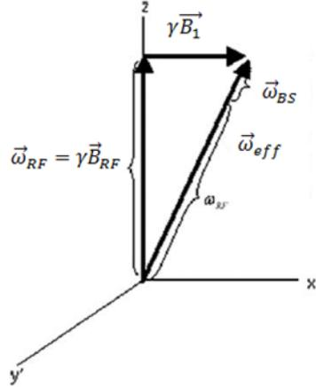
Figure 1.4.1: Illustration of Bloch-Siegert Shift (modified from the Fig.1 in [1]). The  $B_1$  rotating frame rotates at frequency  $\omega_0 + \omega_{RF}$ , and the spins rotate at  $\omega_{RF}$ .  $\omega_{BS}$  is the Bloch-Siegert shift.
