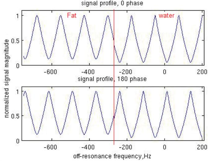
Figure 6.2.1: Profiles of 0 and 180° phase-cycled signals by the proposed G-STFR sequence. These profiles are produced by typical  $T_1$ ,  $T_2$  values of water and fat for demonstration purpose.
