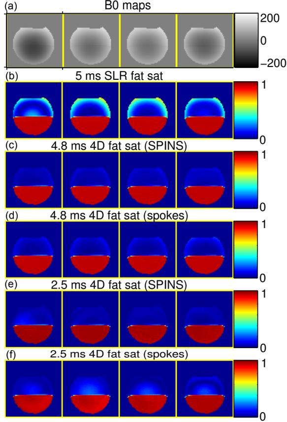
Figure 4.4.3: The  $B_0$  maps and the results of experiment 2, where every third of the axial slices is shown. (a) The  $B_0$  maps (in Hz); (b)-(f) The ratio images by different pulses: (b) 5 ms SLR fat sat pulse, (c) 4.8 ms 4D fat sat pulse with SPINS trajectory or (d) spoke trajectory, (e) 2.5 ms 4D fat sat pulse with SPINS trajectory or (f) spoke trajectory. The ratio images are still the ratio between the images with fat sat and the ones without fat sat, and oil is still on top of water.
