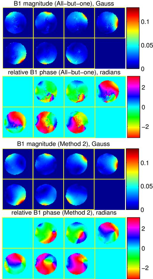
Figure 3.4.9: The resulting  $B_1$  magnitude and phase maps by the two different coil combinations. The  $B_1$  estimates based on the optimized coil combination matrix (bottom two sets of images) have better SNR than the conventional all-but-one approach (top two sets of images).
