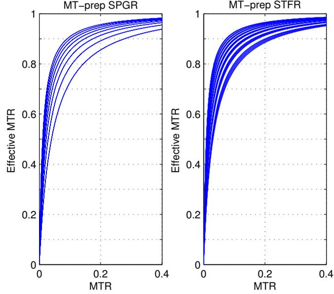
Figure 5.2.2: The plot of the effective MTR in terms of MTR for MTC SSI sequences;  $0.5 \text{ s} \leq T_1 \leq 2 \text{ s}$ ,  $50 \text{ ms} \leq T_2 \leq 200 \text{ ms}$ . It shows that both sequences are sensitive to small magnetization attenuation caused by MT effect.
