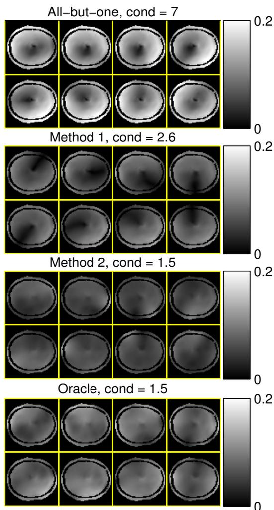
Figure 3.4.5: Magnitude of the composite  $B_1$  maps (masked),  $\tilde{B}_n(\mathbf{r})$ , by different methods, in Gauss. The condition numbers (cond) of each combination matrix are shown on the titles.
