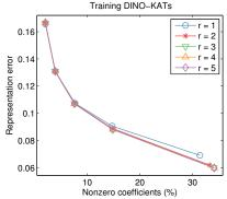
Representation error  $\|\boldsymbol{X} - \boldsymbol{D}\boldsymbol{C}'\|_F / \|\boldsymbol{X}\|_F$  versus sparsity  $\lambda$  for several atom ranks r for  $8 \times 8 \times 5$  space-time patches from (fully sampled) cardiac perfusion images.
