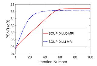
(SNR compared to fully sampled image.) Using  $\|\boldsymbol{z}_m\|_0$  leads to higher SNR then  $\|\boldsymbol{z}_m\|_1$ . Adaptive case is non-convex anyway...
