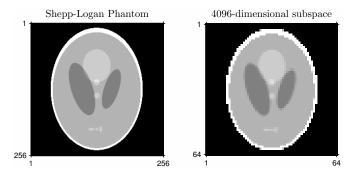
Subspace representation (using pixel basis) is undesirably coarse.
