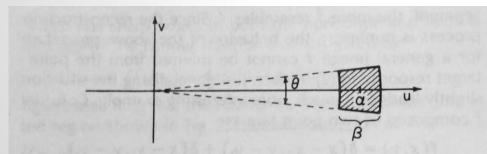
**Fig. 1.** Region of known Fourier-domain data F(u, v) in spotlight mode synthetic-aperture radar. Typically  $\beta \ll \alpha$  and  $\theta$  is quite small as shown.
