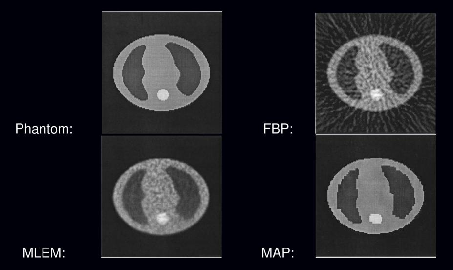
Lee *et al.*, IEEE T-NS, 2002, 300K counts non-convex "broken parabola" potential function and deterministic annealing
