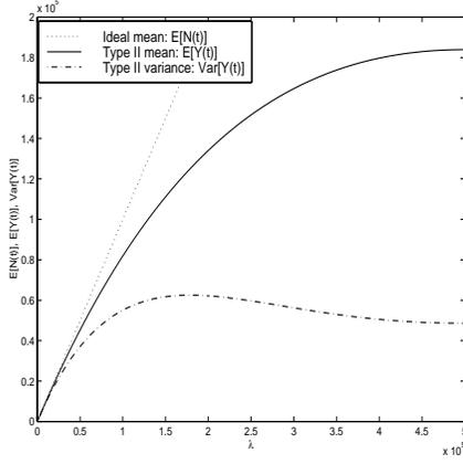
Fig. 1 Mean and variance for paralyzable (type II) systems, with  $t = 1s$ ,  $\tau = 2\mu s$ .
