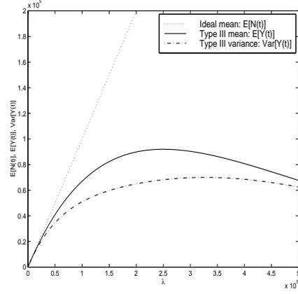
Fig. 2 Mean and variance for type III systems, with  $t = 1s$ ,  $\tau = 2\mu s$ .
