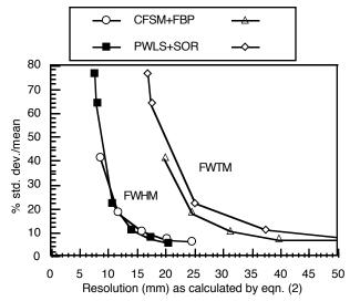
Fig. 7. Background noise vs. resolution as measured by the FWHM and FWTM of a line source in a warm cylinder.
