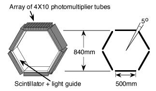
Fig. 1. Geometry of the PENN-PET scanner.
