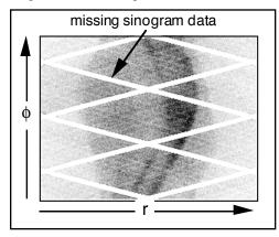
Fig. 2 Missing sinogram data due to 50 detector gaps.
