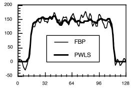
Fig. 4. Transverse line profiles through the center of the images (shown above) reconstructed by FBP and PWLS. Pixels are 2 mm.
