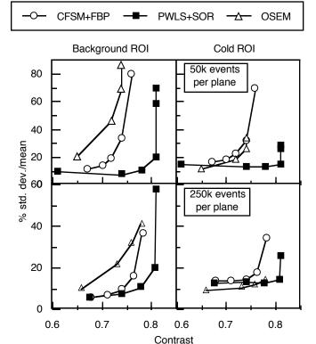
Fig. 8. Contrast vs. noise for two different imaging conditions. OSEM (without proper system model) is also included.
