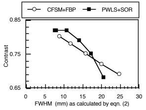
Fig. 9. Contrast vs. resolution as measured from a cylinder with a hot line source, a warm background and a cold insert.
