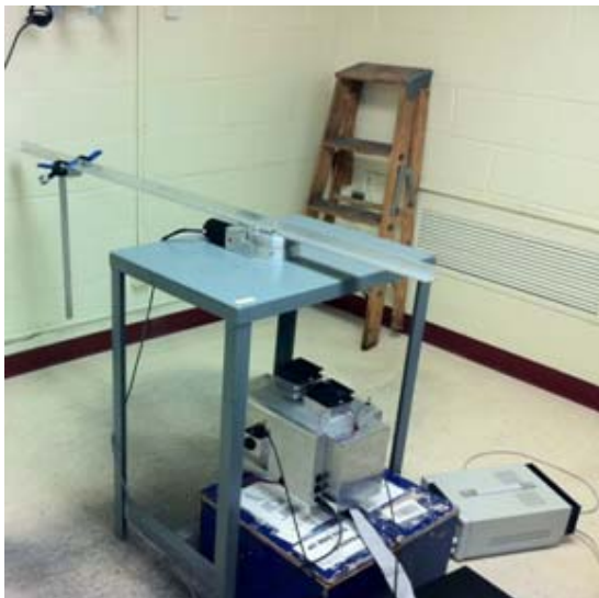
Fig. 2. A computer controlled actuator arm is used to control the position of the source with known motion. The Polaris system is positioned directly underneath the actuator pivot point, and the source is placed at the bottom of the actuator arm in-plane with the detector system.
